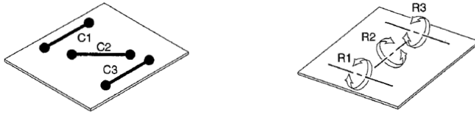
Figure 2.10: A constraint-space picture and a freedom-space picture describe the same design from opposite sides. Screw theory writes this complement as reciprocal twist and wrench spaces.
